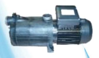
Multi-cellular pump for use with automatic cleaners. Pump body in noryl with fibreglass. Shafts and screws in Stainless Steel AISI-316. Mechanical seal in S.S. and Graphite. Motor: protection IP-55, isolation class F, non-stop operation, 2850 rpm
